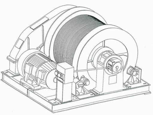
The gearbox is two-gear, or alternatively three-gear with frontal cogwheels. Fast-speed gearing has diagonal cogs, the slow-speed gearing has direct cogs. Cog and bearing lubrication is solved by wading (oil spraying).
