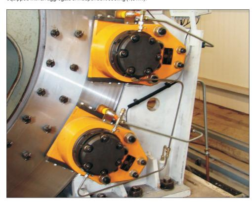
The power part of the brake system is formed by two brake stands each of which bears one or two brake units HPB200(see the separate catalogue sheet), depending on the type of the machine, or alternatively at customer's request, brake units Svendborg BSFG-408A or Zgoda SH100B. In disc brake units the braking power is created by sets of preloaded disc springs, while the brake release is ensured hydraulically.
